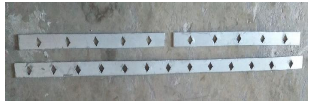
Figure 1: Diamond-cut single and separated inserts
